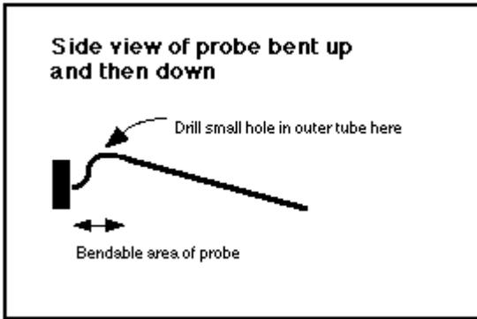
4. Bend 1/4" probes no tighter than a 1" radius. Bend 1/2" probes no tighter than a 3" radius.
