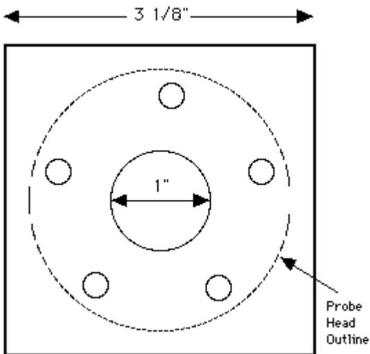
flange. NOTE THAT THE HOLE PATTERN IS NOT SYMMETRICAL IN EITHER THE FLANGE, GASKET OR PROBE. THE SPACE BETWEEN TWO OF THE HOLES IS A LITTLE LARGER THAN THE SPACE BETWEEN THE OTHER HOLES!
