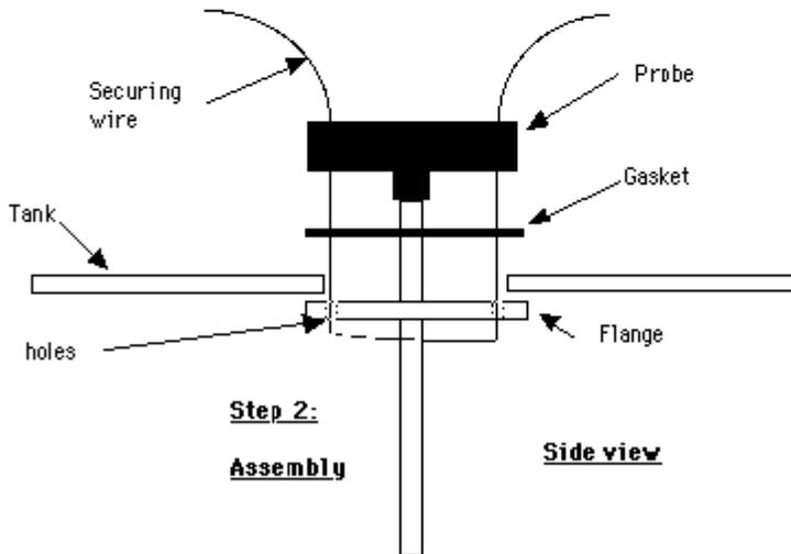
1. Locate internal flange. Note notch in outer edge. Thread a thin wire (like safety wire) or string at least 24" long through two non-adjacent holes in the flange. See drawing on page 4. Set the flange aside for now.
